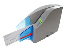
• Slide the item(s) up to the line on the body of the scanner as indicated below. The status LED light will turn 'Orange' when an item is detected.
