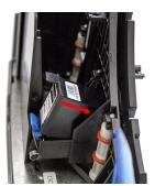
• Then, push down on the rear of the cartridge until it 'clicks' or snaps securely into position.
