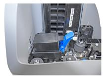
• The cartridge should appear tilted at a slight angle when it is fully seated. Reinstall cover.
