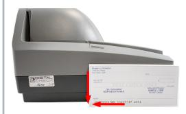
• Slide the item(s) up to the line on the body of the scanner as indicated below. The status LED light will turn 'Orange'.
